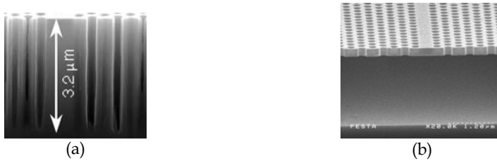
Fig. 3. Scanning electron microscopy images of (a) InP-based substrate-like and (b) GaAs-based membrane-like planar photonic crystals [(a) Ferrini et al., 2002a; (b) Sugimoto et al., 2004].
