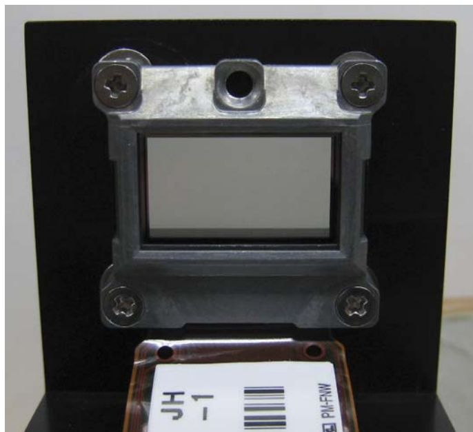
Fig. 1. Photograph of a liquid crystal - spatial light modulator (LC-SLM). The modulator is an LCD panel (L3D07U-81G00 Seiko Epson Corp.)
