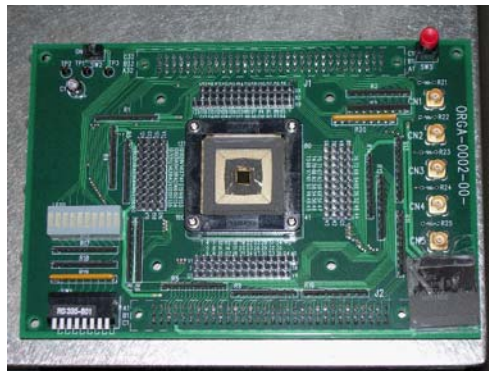
Fig. 6. Photograph of an ORGA-VLSI board with a fabricated ORGA-VLSI chip. The ORGA-VLSI was fabricated using a 0.35 \mu\text{m} three-metal 4.9 \times 4.9 \text{ mm}^2 CMOS process chip. The gate count of a gate array on the chip is 68. In all, 340 photodiodes are used for optical configurations.
